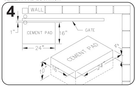
O If no concrete surface exists to attach the gate operator to, make a cement pad 16" X 24" X 10". The cement pad should be at least 6" in depth and extend below frost line. If it is desirable to elevate the gate operator it may protrude 4" or more above ground as shown. Place the shortest pad edge even with the driveway edge. Place the longer edge of the pad 1" away from the gate.
